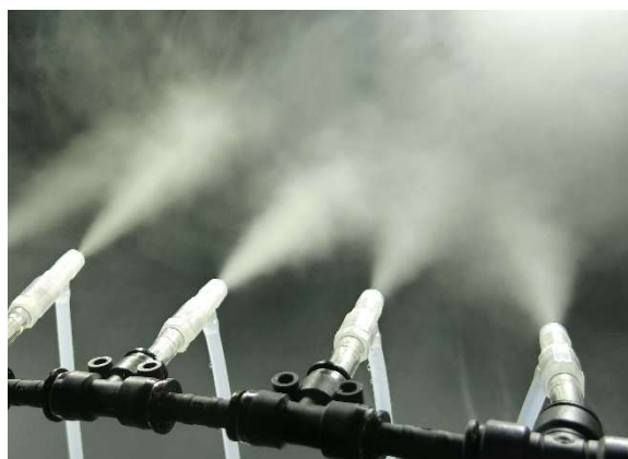
[5.2] Connected spraying (with use of some commercial parts)
